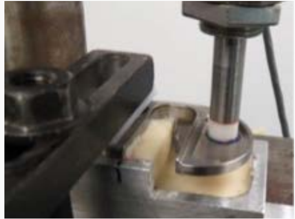
Figure 5: Tibial tray fatigue strength test setup.
