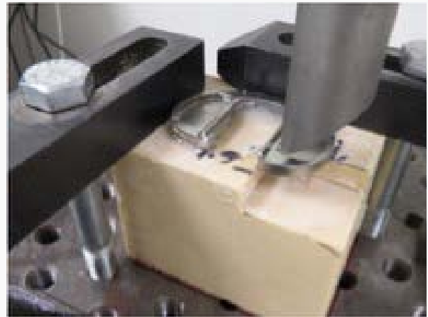
Figure 6: Tibial fixation test setup.
